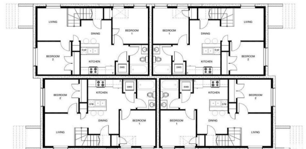
BASEMENT SUITE FLOOR PLAN 548 SQ. FT. / UNIT
